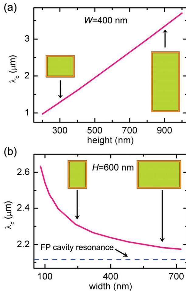
**Figure 2.** Resonant wavelength ( $\lambda_c$ ) as a function of the rod height (a) and rod width (b). The relative geometries of the cross-sections of the rods are depicted in the insets. It is shown that when the rod width is simply increased,  $\lambda_c$  approaches the resonant wavelength of an FP cavity with  $H = 600$  nm and  $W = \infty$ .
