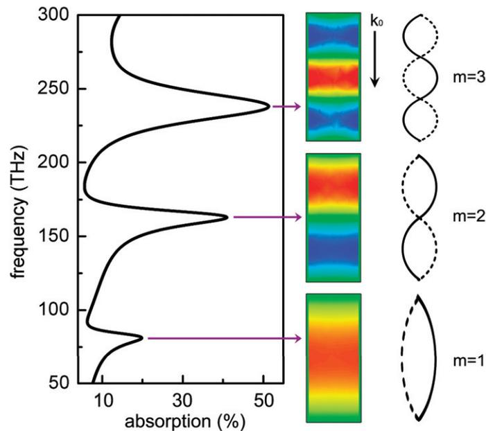
**Figure 3.** Absorption spectrum (left) and internal  $E$ -field distribution at the resonant frequencies (center) of NRods. (Right) Schematic diagram of the cavity resonances at corresponding orders of the resonances. Simulation parameters:  $W = 400$  nm,  $H = 1000$  nm,  $D = 15$  nm,  $a = 1000$  nm and  $n = 1.56$ .
